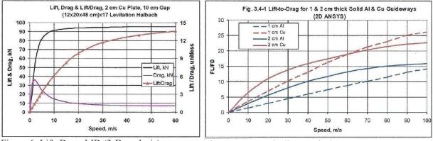
Figure 6: Lift, Drag, LID (3-D analysis) Figure
