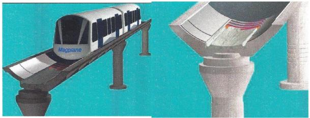
motor winding directly below the vehicle.
