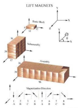
Figure 5: Lift Pad magnetic structure built from magnetized unit blocks
